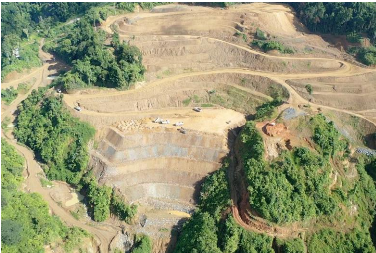
1 The Balabag Project's Waste Rock Dump (WRD) landscape before the progressive rehabilitation in 2021.
