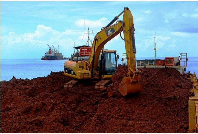
**Fully loaded.** AMVI loads shipments of approximately 55,000 wmt of high-iron/low-nickel ore every three to four weeks with shipping rates expected to ramp-up to 2.5 million wmt per year in 2015. (In photo): an excavator compacts nickel ore on a barge, which will then transport the cargo to a bigger vessel (in background).
