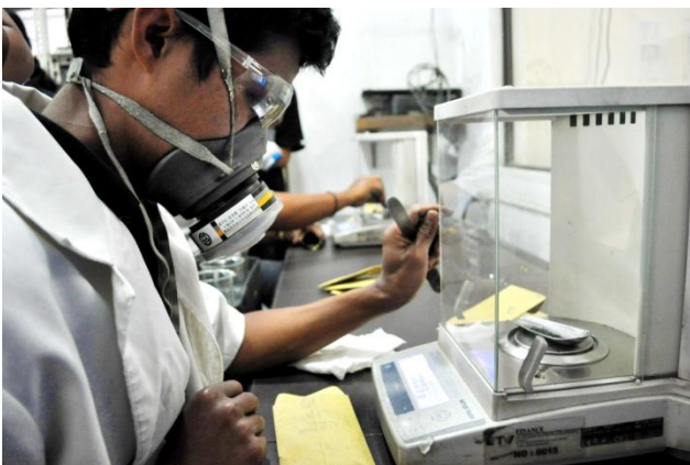
1-2 Mineral Analysis. (Top): The ore samples are subject to extremely high temperatures to determine its mineral content. TVIRD chemists are mandated to wear protective equipment like full-face masks to protect them from gas-fire spatters. (bottom) Respirators are compulsory for chemists, even when weighing materials prior to analysis.
